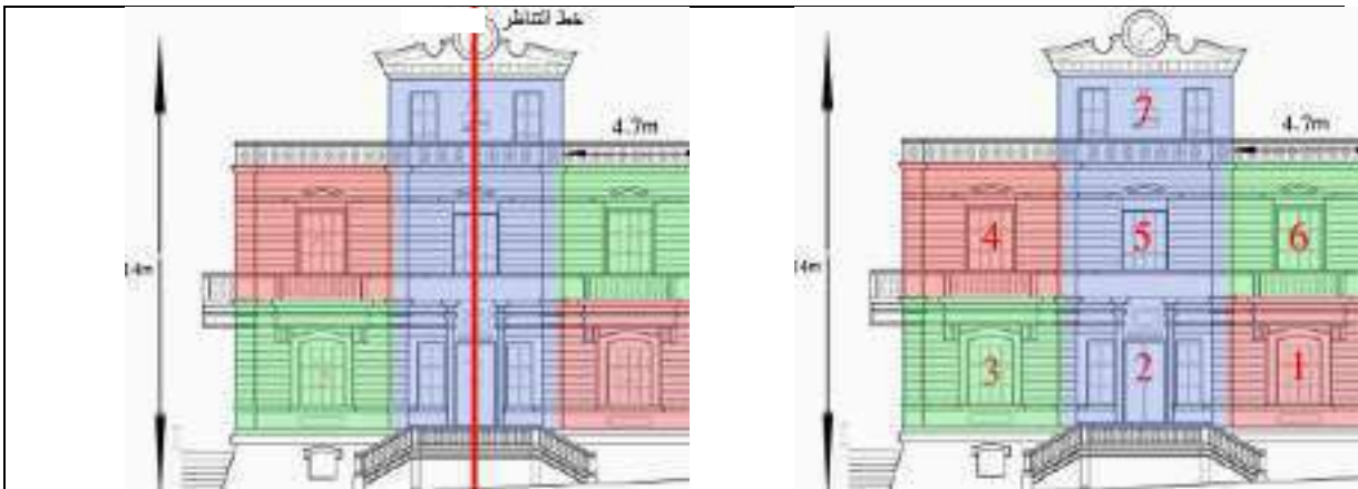
Figure (3-17) Analysis of the main western facade of the immigration and passport building in old Aleppo (Arch pillars, 2022).
